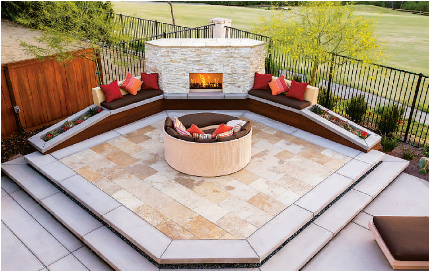
A two-step cantilevered elevation serves as an outdoor living room with a ventless fireplace veneered with LedgeStone and flanked with polished concrete benches. The daybed in the center is a good place to relax and enjoy the view.
